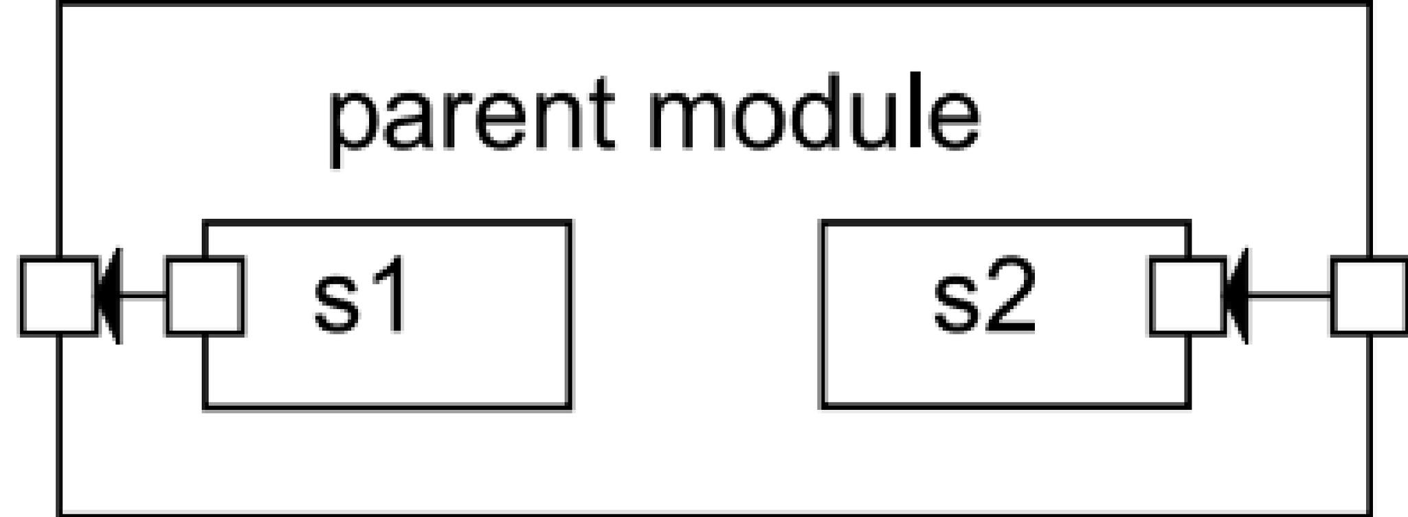
Submodules connected to the parent module
