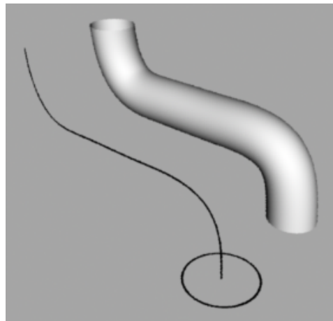
Figure 17: Sweep Object (left: Curves, right: Resulting Swept Surface)
