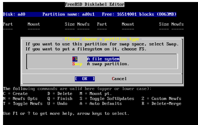
Figure 2-22. Choisir le type de la partition racine
