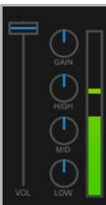
The VOL slider controls the volume of the selected channel. The GAIN knob can be used to apply extra amplification to a quiet song, which can be used to match its volume with the song in the other channel. The HIGH, MID, and LOW knobs perform equalization on the channel, reducing or increasing high, mid and low frequencies accordingly.
