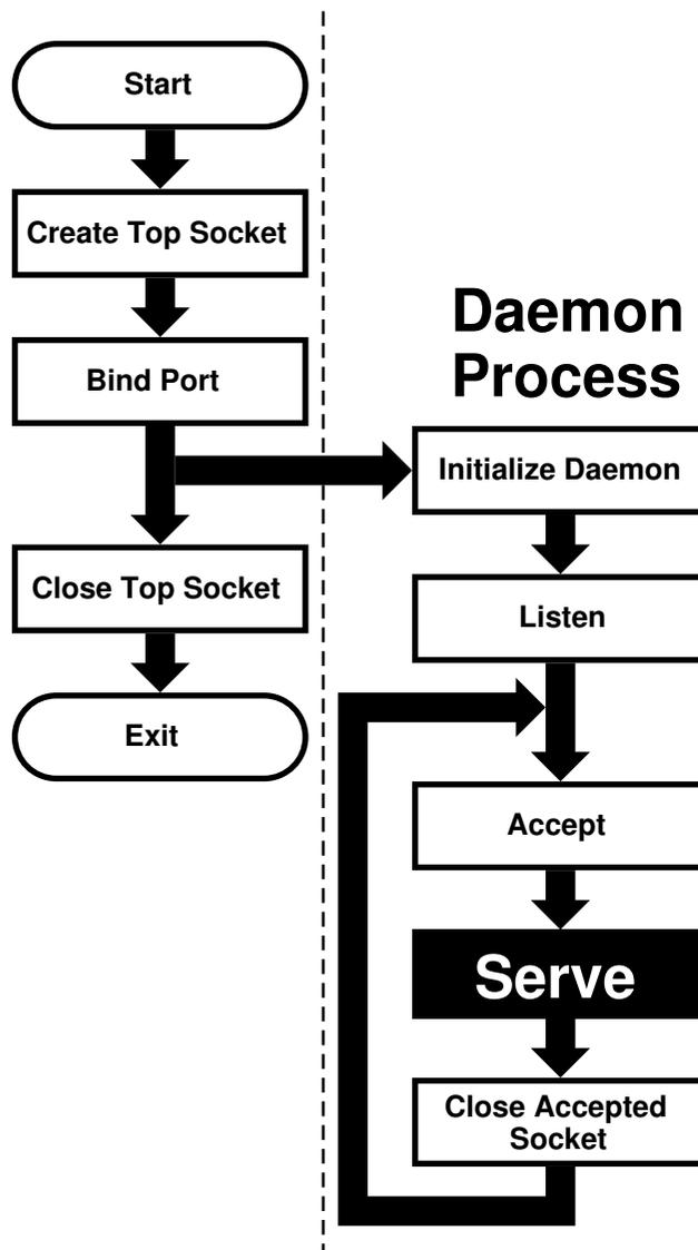
This flowchart is good for *sequential servers*, i.e., servers that can serve one client at a time, just as we were able to with our *daytime* server. This is only possible whenever there is no real `E` conversation`F` going on between the client and the server: As soon as the server detects a connection to the client, it sends out some data and closes the
