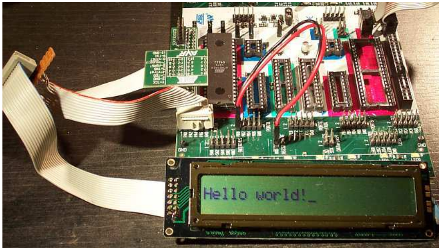
Figure 9: Wiring of the STK500
